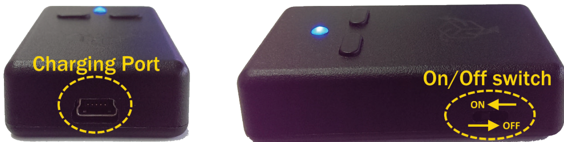
Figure 2. Head Tracker charging port & power switch
