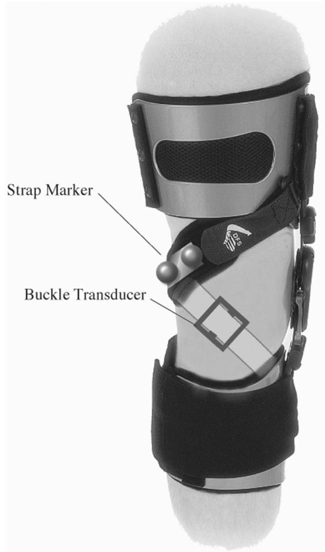
**Figure 2.** The orientation of the dynamic force strap at the knee joint line was determined by using a marker set that consisted of a pair of reflective markers on a plate. The marker set was aligned with the strap at the lateral aspect of the knee at the level of the joint line.
