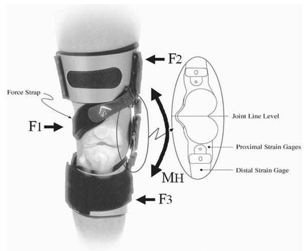
**Figure 1.** Schematic of the Generation II Unloader brace on a limb with the upper and lower cuff supports and the Dynamic Force Strap.  $M_H$  represents the valgus moment contribution due to the hinge.  $F_1$ ,  $F_2$ , and  $F_3$  represent the three-point bending forces generated by the tension in the force trap. The isolated view shows the lower tibial support with a single strain gauge attached at level 1 and two strain gauges attached at level 2.
