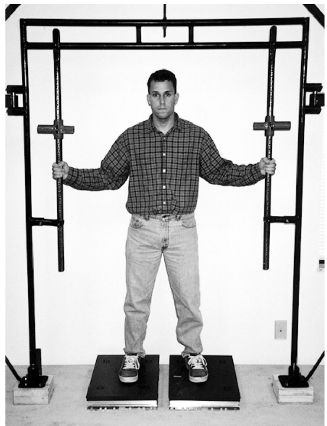
Fig. 1. Isometric strength-testing apparatus.
