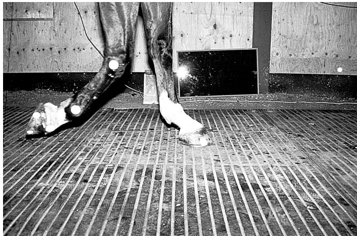
Fig. 3.9 Horse stepping on a force plate during data collection.
