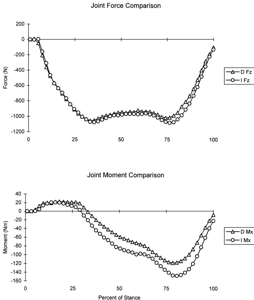
Fig. 1. Representative ankle joint forces (N) and moments (N m) (subject 1, trial 6) measured directly (D) with the PY-6 transducer and through inverse dynamics (I), vs. percent of stance phase.
