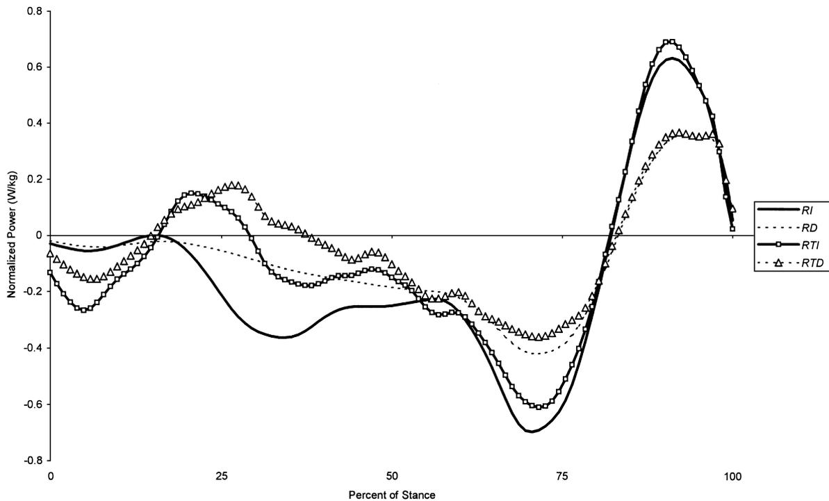
Fig. 2. Normalized sagittal ankle joint power (W/kg) vs. percent of stance phase, ensemble average of all subjects, comparison of each analysis technique: R = rotational power only, RT = rotational plus translational power, D = directly measured ankle kinetics, I = inverse dynamics-calculated ankle kinetics. Comparisons are made of each new method vs. RI, the standard method.
