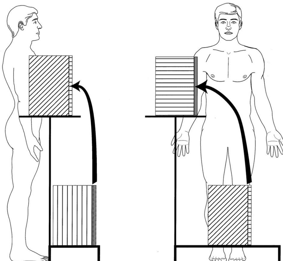
Fig. 1. Front and side views of experimental setup. A 9.4 kg frame box was lifted from a position in front of the body to a stand  $60^\circ$  to the right of the subject.
