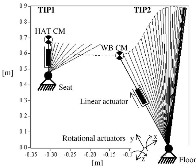
Fig. 1. Schematic representation of the two TIP models employed for the description of STS. TIP1: before seat unloading. TIP2: after seat-off. The sign convention for the actuators is also indicated.
